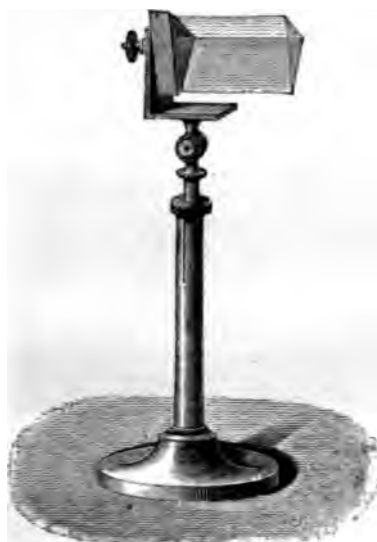
FIG. 32.—Prism mounted on a stand.
